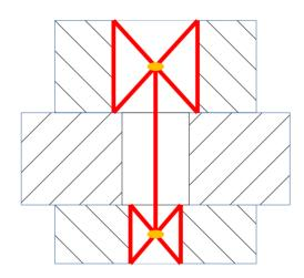
Multi point element, several-several. Surface-Surface. *E.g. inside thread to inside thread.*
